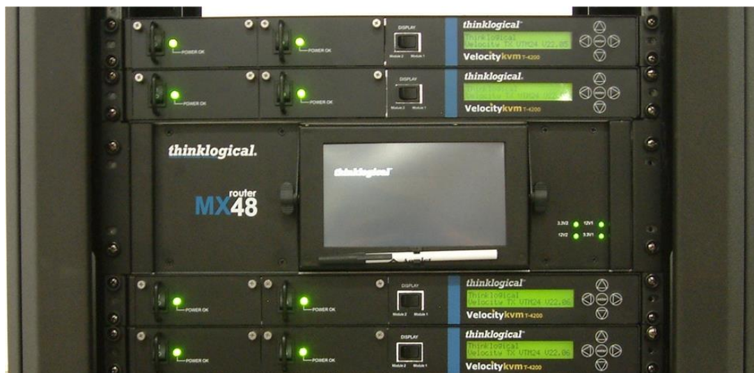
Figure C4: Rack-Mounted Router with touch screen mounted in a rack with Thinklogical® VelocityKVM T-4200 units.
