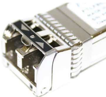
Figure 12a: SFP+ latch closed
