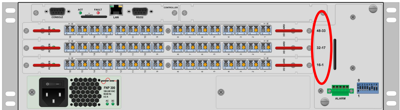
Figure 9: Input / Output Port Numbering on the MX48
