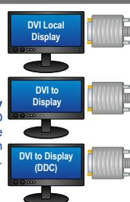
**STEP 6:** Connect an optional local monitor to the transmitter's DVI LOCAL DISPLAY port.
