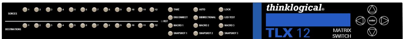
The Button Panel, located on the front of the TLX12, provides Matrix Switch control via the RS232 port's API interface. The following pages provide a functional description of each of the 36 buttons.
