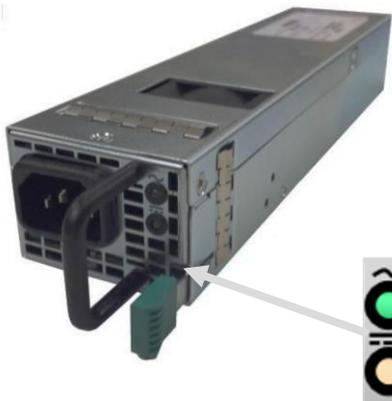
The TLX12 Power Supply is a high efficiency, 650-watt supply (100-240VAC, 50-60Hz input) with a **12V main output** and a **12V standby**. The supply includes an internal cooling fan, status LEDs on the outer panel and over-current, over-voltage and over-temperature protection. The supply is NOT hot pluggable. (See pg. 18 for the *Poweroff* procedure.)
