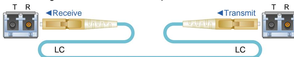
*Thinklogical recommends SX+ Laser Enhanced Fiber-optic Cable, 50 or 62.5 microns, terminated with LC type connectors.*
