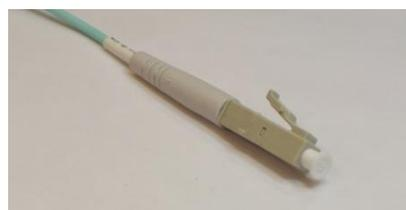
*Dust cap installed on the ferrule.*
