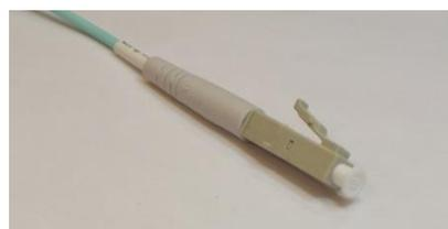
Dust cap installed on the ferrule.
