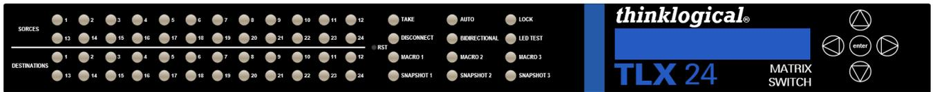
The Button Panel, located on the front of the TLX24, provides Matrix Switch control via the RS232 port's API interface. The following pages provide a functional description of each of the 60 buttons.
