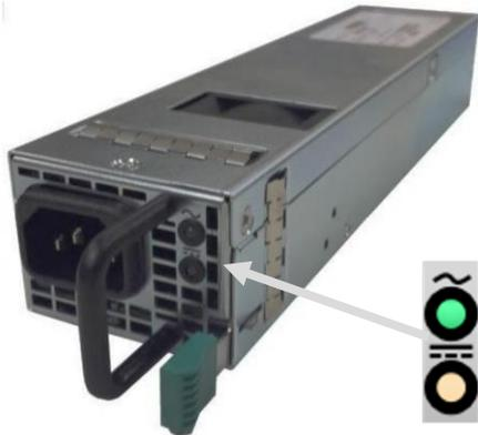
The TLX24 Power Supply is a high-efficiency, 650-watt supply (100-240VAC, 50-60Hz input) with a **12V main output** and a **12V standby**. The supply includes an internal cooling fan, status LEDs on the outer panel and over-current, over-voltage and over-temperature protection. The supply is NOT hot pluggable. (See pg. 19 for the *Poweroff* procedure.)
