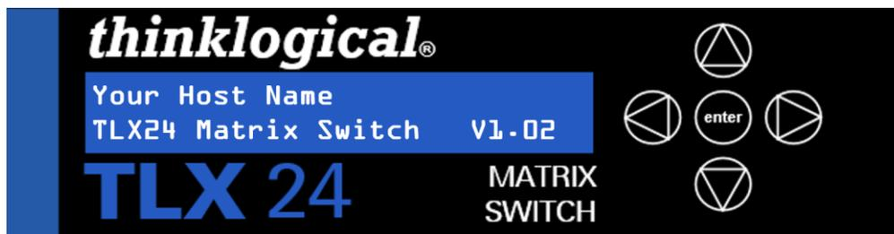
Your chosen *Host Name* is listed on the first line of the display. The model and software version (VX.XX) of the unit are displayed on the second line.
