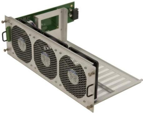
The TLX320 uses 3 DC fans located in one modular, hot-swappable fan tray designed for easy replacement without interrupting system functionality. The Fan Tray introduces air into the chassis through air baffles within the chassis. This cools the vertically mounted I/O Cards, the Controller Cards and the backplane.
