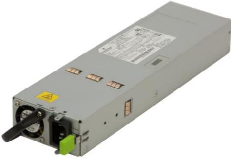
The dual, redundant power supplies ensure continuous, uninterrupted power. The supplies are current sharing which means the supplies share the load equally. If a power supply fails, the redundant power supply can support the entire current load of one fully populated card cage.
