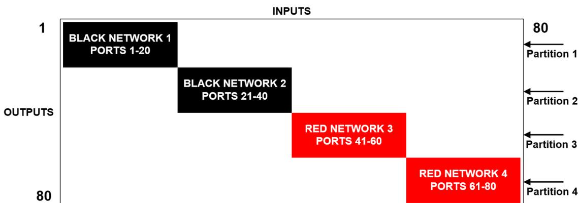
*Four partitions set up for secure routing and extension applications. Signals are only capable of transmitting and receiving within a single partition and not across partitions*
