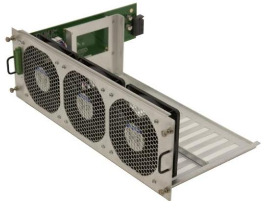
**ALARMS:** The Fan Tray is equipped with an annunciator port for system alarms that can be configured to trigger an external control system. The dry alarm contacts are *Normally Closed* when unpowered, *Normally Open* when powered (OK condition) and *Closed* for an alarm condition.
