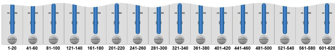
The TLX640 configuration can have a minimum of one I/O Card (20 x 20) and a maximum of 32 I/O Cards. Each TLX640 I/O card contains 20 ports. When fully configured, the TLX640 contains 16 I/O cards in the Upper Card Cage and 16 I/O cards in the Lower Card Cage. The 32 I/O cards provide a total of 640 Optical Input/Output connections described as Ports 1-640.
