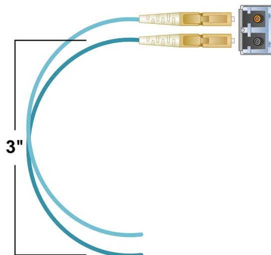
*Thinklogical recommends SX+ Laser Enhanced Fiber-optic Cable, 50 or 62.5 microns, terminated with LC type connectors.*
