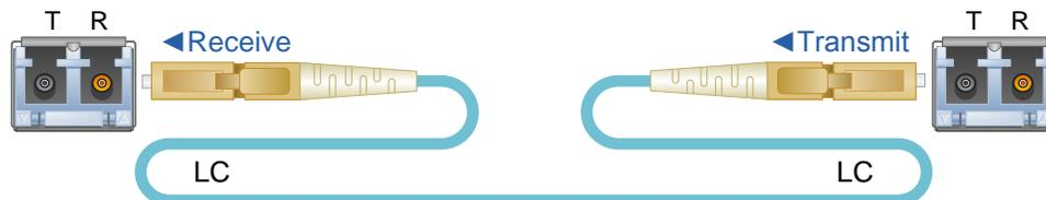
**Handling Fiber-optic Cable:** Unlike copper cabling, fiber-optic cable requires special handling. A small speck of dust or a scratch to the ferrule tip (the end of the connector) can attenuate the optical signal, rendering the cable inoperable.
