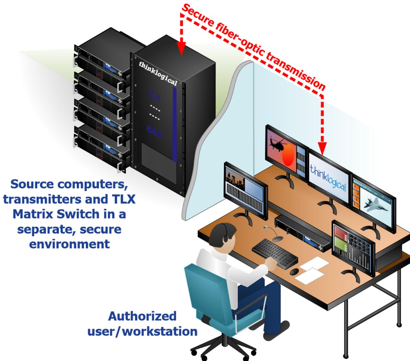
Thinklogical's TLX, VX and MX Matrix Switches use two methods for secure routing. One is known as **Restricted Switching** and the other is known as **Partitioning**. These methods can be deployed singularly or jointly, depending on security requirements.
