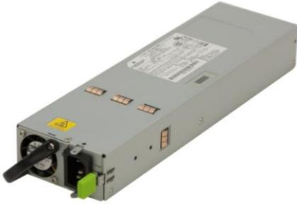
The dual, redundant power supplies for each card cage ensure continuous, uninterrupted power. The supplies are current sharing which means the supplies share the load equally. If a power supply fails, the redundant power supply can support the entire current load of one fully populated card cage. Although the TLX640 functions properly with one Power Module per card cage, Thinklogical recommends that both modules be used, preferably connected to independent power sources for redundancy.
