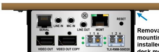
Removable mounting brackets installed for under-desk mounting.
