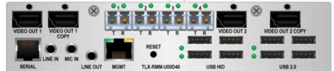
**VIDEO EXTENDER MODULES** (All support DisplayPort 1.2. "D" supports HDMI 1.4, "E" supports HDMI 2.0)
