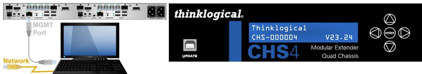
2. Using the down arrow, scroll to the module's **Card Slot**. (KVM Modules occupy Cards 2 and 4).
