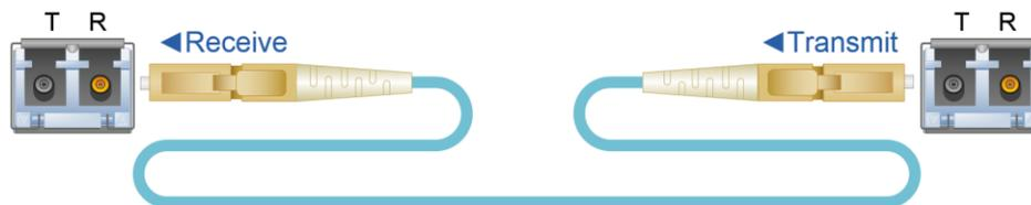
**Handling Fiber-Optic Cable:** Unlike copper cabling, fiber-optic cable requires special handling. A small speck of dust or a scratch to the ferrule tip (the end of the connector) can attenuate the optical signal, rendering the cable inoperable.
