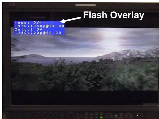
*Flash Overlay on-screen display of output settings*
