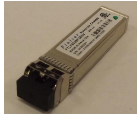
Dust plug in unused SFP+
