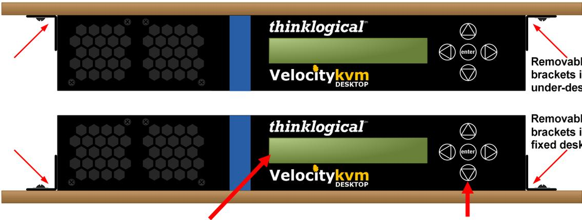
Removable mounting brackets installed for under-desk mounting.
