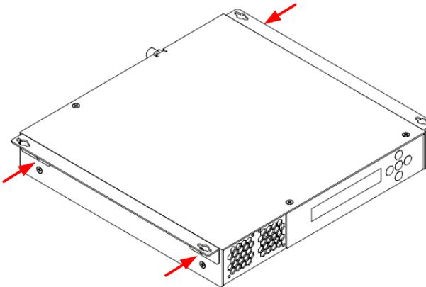
The included mounting brackets can be installed for fixed desktop mounting or under-desk mounting simply by removing two screws per bracket.
