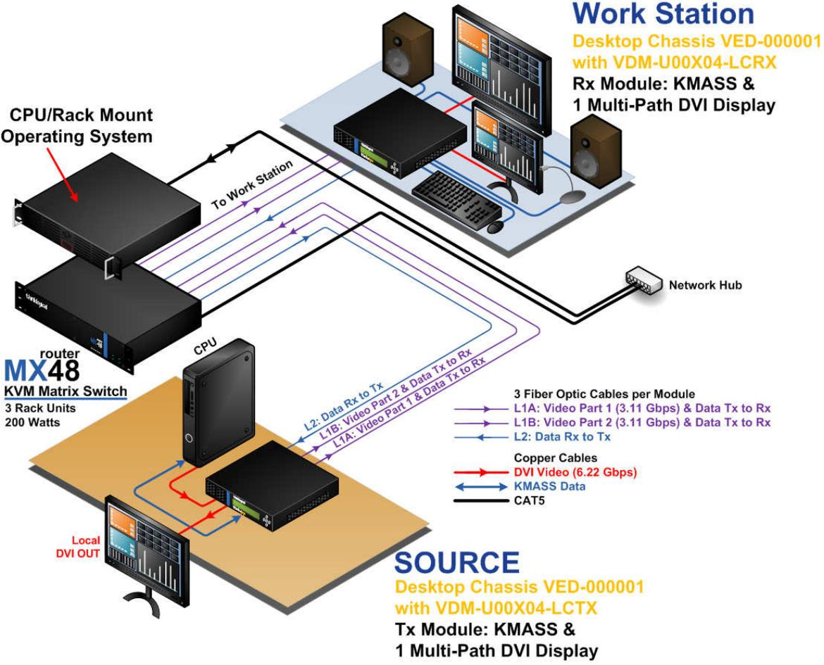
*Multi-Video Path Tx Module to Multi-Video Path Rx Module Application*
