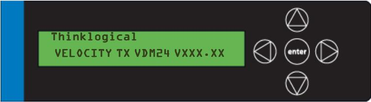
The company name is listed on the first line of the display. The model and software version (VXX.XX) of the unit is displayed on the second line. In the front panel menus, the word **card** is used in place of **module**, but refers to the same devices described elsewhere throughout this document.
