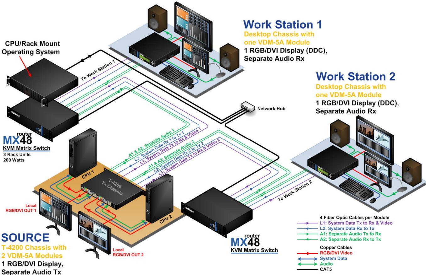
**Dual RGB/DVI/Separate Audio Tx Modules (T-4200 Chassis) to RGB/DVI/Separate Audio Rx Modules in two Desktop Chassis**
