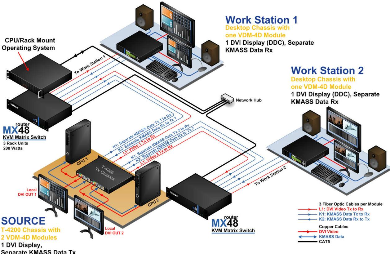
**Dual DVI/Separate Data Tx Modules (T-4200 Chassis) to DVI/Separate Data Rx Modules in two Desktop Chassis**
