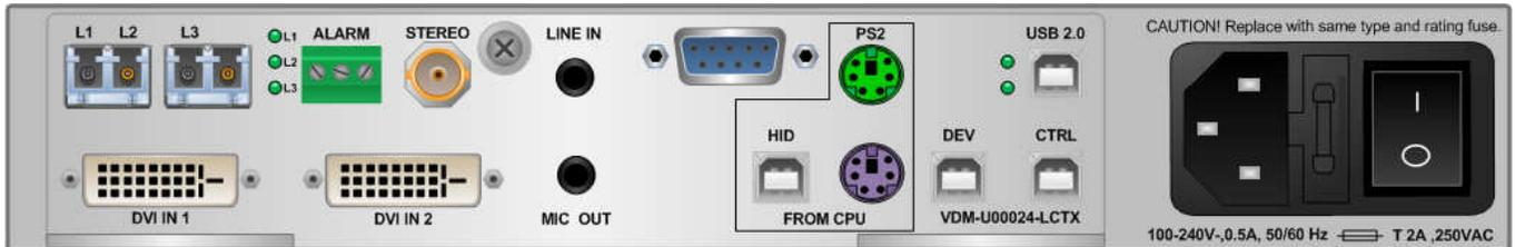
All physical connections to the VelocityKVM Desktop use industry-standard connectors. VelocityKVM Desktop is shown with a Velocity 24 TX Module (VDM-U00024-LCTX) installed.
