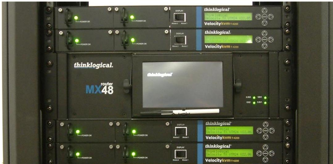
**Figure C4:** Rack-Mounted Touchscreen displayed in a rack with Thinklogical® VelocityKVM T-4200 units
