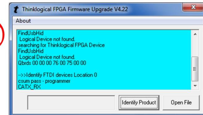
**STEP 10:** Select *Open File* and repeat the previous steps to update the RX modules. Be sure to move the USB cable to the Receiver's Update Port.
