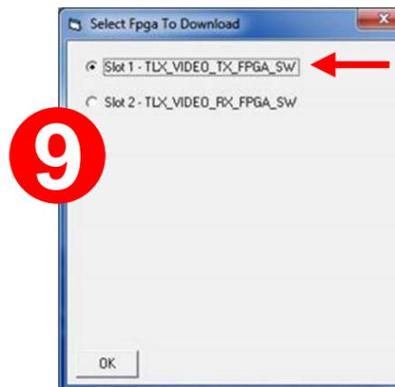
**9 STEP 9:** You will see a window similar to this, depending on how many slots in the chassis are occupied (2 in this example). As shown, there is one firmware option for each of the TLX Video modules.
