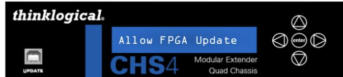
**5 STEP 5:** Connect a USB cable from the front panel of the CHS-2 or CHS-4 chassis to the CPU. (When connecting Thinklogical equipment to your PC for the first time, it may take a few moments for Windows to correctly install the required drivers.) Open the Windows *Device Manager* to check that all drivers are installed correctly.
