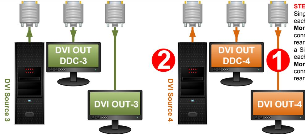
**STEP 1:** Connect one end of a Single-Link DVI-D cable from each **primary DVI Output Monitor** to the DVI OUT DDC connector on the VDA Splitter's rear panel. Connect one end of a Single-Link DVI-D cable from each **secondary DVI Output Monitor** to the DVI OUT 2 connector on the VDA Splitter's rear panel.
