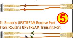
Multi-Mode fiber can be up to 1000 meters in length. Single-Mode fiber can be up to 40 kilometers.
