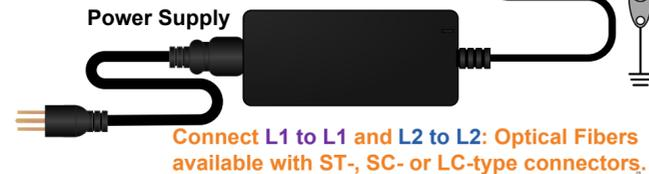
**STEP 4:** Connect your fiber optic cable, up to 1000 meters (available through *Thinklogical™*) between the Transmitter and Receiver Units. Do not kink or pinch the cable and be sure to keep all bend radii to no less than 3 inches.
