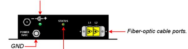
The status LEDs near the USB port on the Tx and Rx units are used to indicate the status of connections to the extender.
