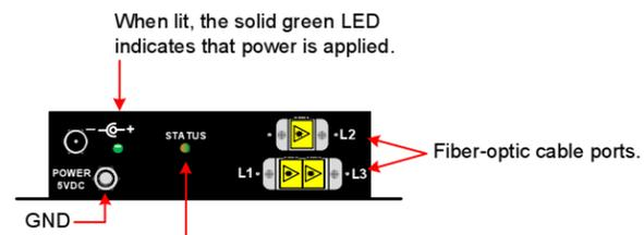
The status LEDs on the Tx and Rx units are used to indicate the status of connections to the extender.
