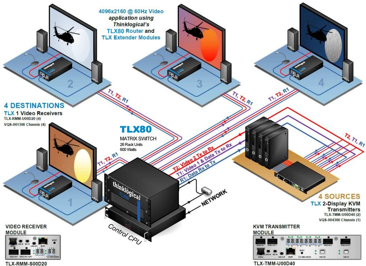
Figure 2a. Typical TOE TLX80 Matrix Switch
