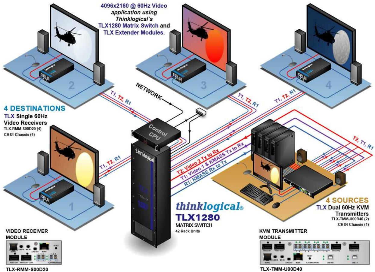
Figure 2a. Typical TOE TLX1280 Configuration
