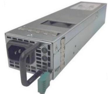
Although the switch functions properly with one power module, **Thinklogical recommends that both modules be used, preferably connected to independent power sources, for redundancy.** Additionally, the hot-swappable feature allows easy replacement of a module without interrupting the Switch's system functionality.
