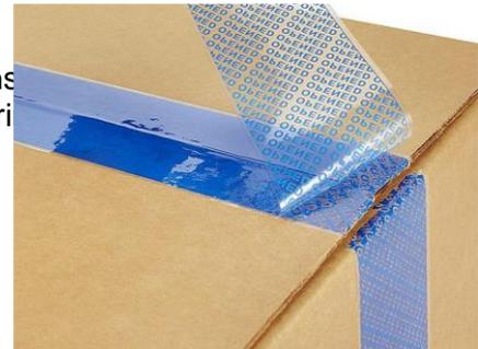
The second type is a striped tape used to seal an open seam on the box. This type of tape cannot be resealed once the box has been opened.
