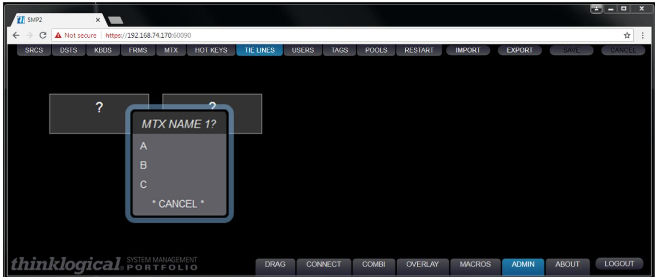
Once the Switches are named, right click within an icon to select a tie line for either direction. Selecting NEW DUPLEX will create a bi-directional tie line using the T and R of the same SFP. Port numbers can be specified in the white fields in each Switch icon. Click **SAVE** to preserve changes.
