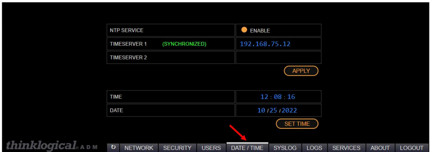
**NTP SERVICE** – Enabled: Network Time Protocol client periodically requests timing information from a NTP server. The client synchronizes to the server every 64 seconds minimum, 1024 seconds maximum.
