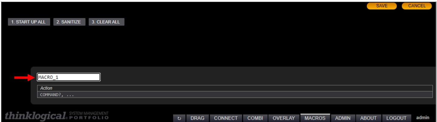
When choosing **FROM SCRATCH**, an Action line appears below the macro's name. Left-click on **COMMAND** and a drop-down menu appears. Here Actions, Sources and Destinations are defined manually. For example, select **CONNECT** as below.
