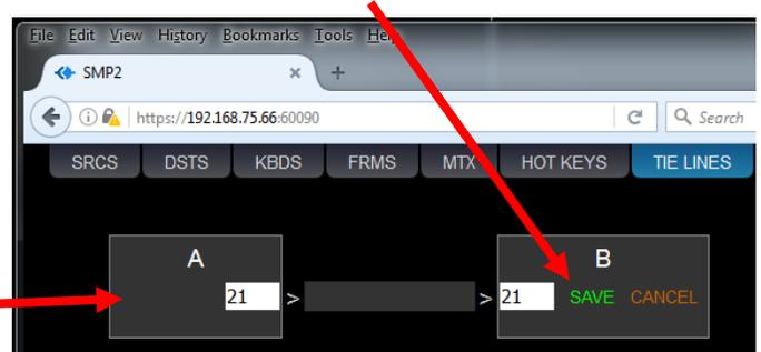
Add tie lines to as many Switches as needed. After the tie lines are created, users may click on them for a new menu: CLEAR, DELETE, AUTO, \*MANUAL\*. Selecting AUTO is required for the SMP3 to automatically use an available tie line when making routes. The \*MANUAL\* selection is used when the tie line is to be used by a third-party control system (such as AMX or Crestron, etc.).
