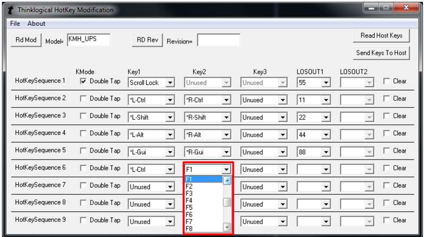
By left-clicking on the **LOSOUT1 drop-down menu**, users can select from a list of hex values, so that pressing *L-Ctrl* and *F1* will execute the function associated with that value.
