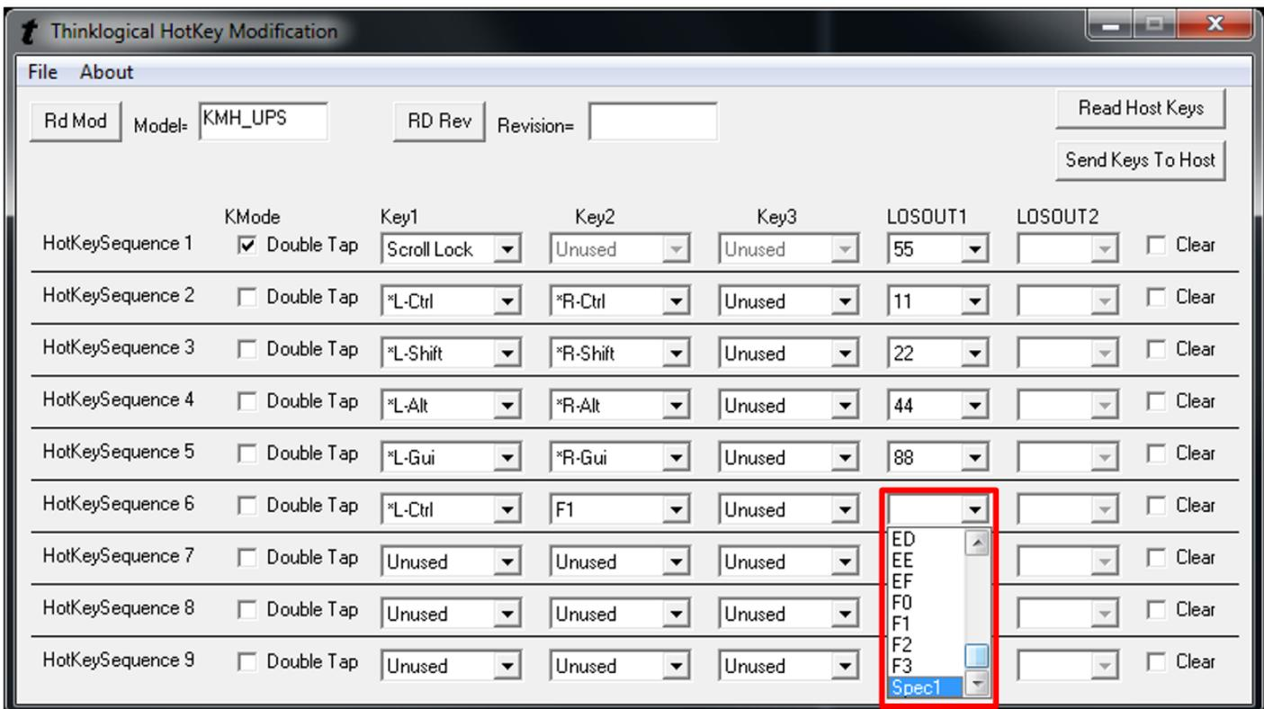
By selecting *Spec1*, the value in LOSOUT2 will automatically become *Rd Kb* (Read Keyboard), meaning it will “read” the next thing typed. **The user must now enter a non-hex numerical value, which will become an action associated with *L-Ctrl* and *F1*.** To clear the entries, click in the *Clear* box to the right.
