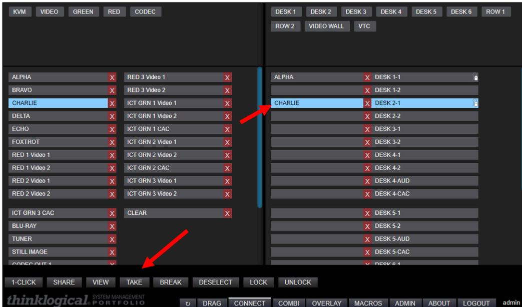
Destinations with active sources will show the names of those sources on the left side. Hovering the cursor over a source or destination will highlight in orange any connections involving that source or destination. Clicking on **X** will break that connection.
