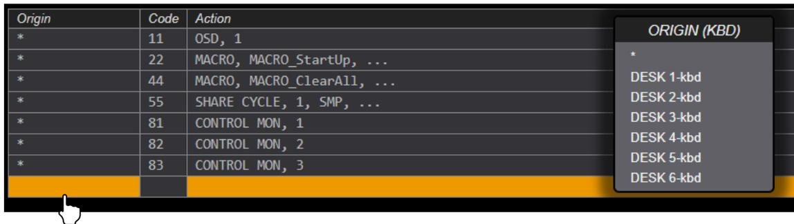
Code: Left-click within the Code field. Type in a hexadecimal key combo as shown below. (In this example code '88' was chosen for a new hotkey function.)
