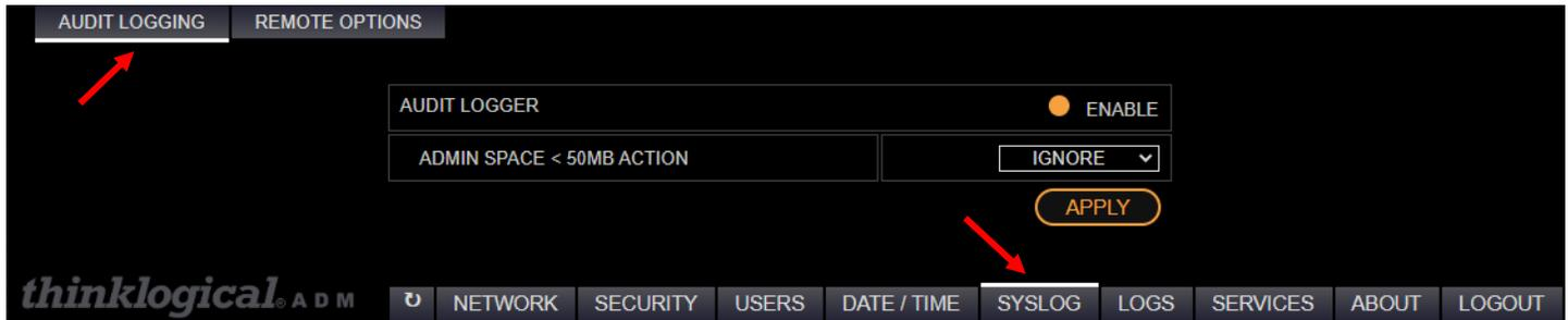
**AUDIT LOGGER** – A security relevant log providing documentary evidence of potentially suspicious events: authentication, changing file permissions, terminating a process, creating a network connection.
