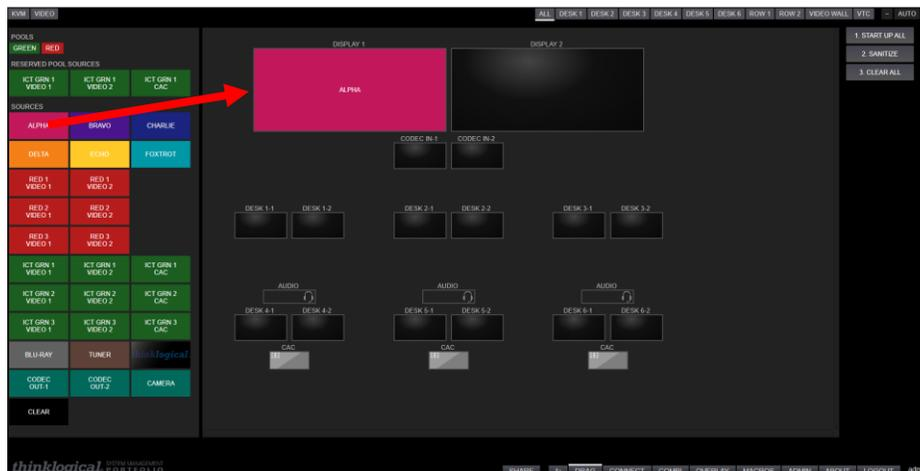
A sample configuration is graphically depicted above in the Drag & Drop GUI, with Sources on the left, Destinations on the right, and Macros on the bottom. Connections can be made or changed simply by clicking on an icon and dragging it to a desired location. Macros can be executed with a single click.
