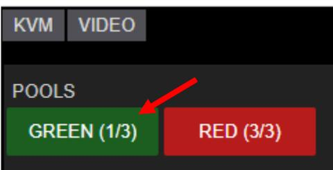
Example: Pools have been created and available (none are currently Reserved here). Note that the POOL icon takes the color of the first Source in the POOL for convenience. Note also in this example the (1/3) indication. This shows there is one Source left (available) out of a total of three.
