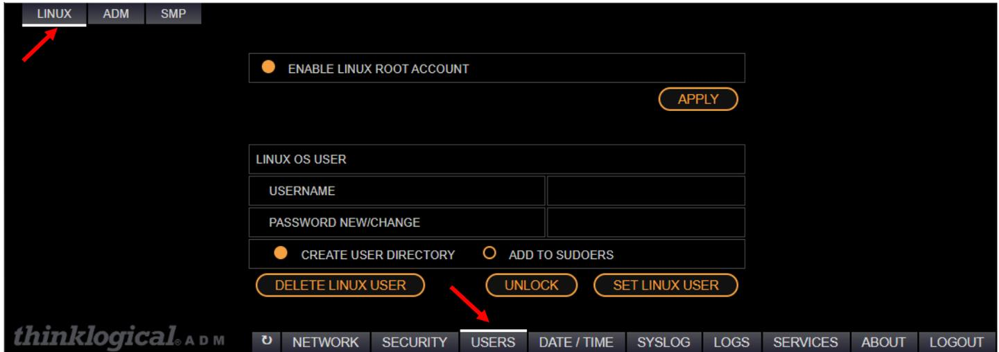
**ENABLE LINUX ROOT ACCOUNT** – Enables / disables ROOT access via SSH and Serial Console port.
