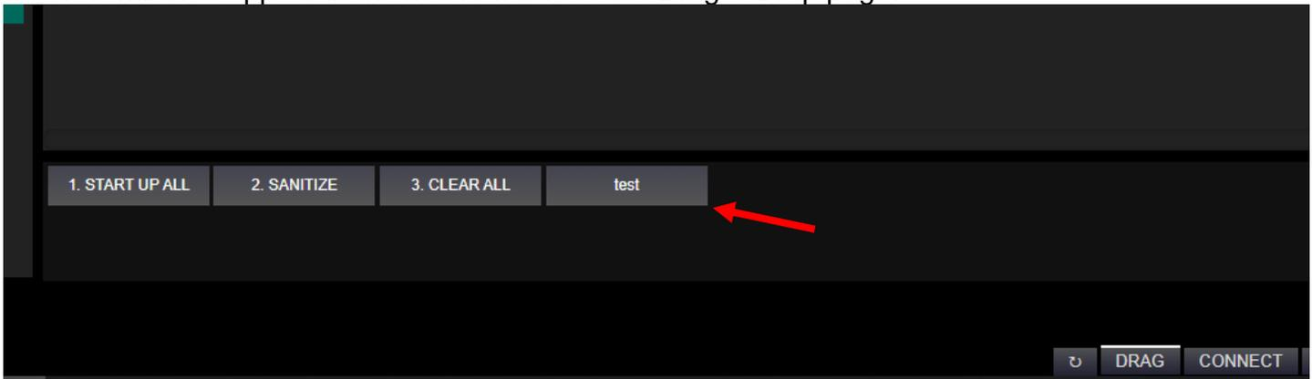
To add the Macro to the Destinations frame, add the prefix "MACRO\_" and the X, Y, W, H parameters. You can also specify an Alias and a color here.
