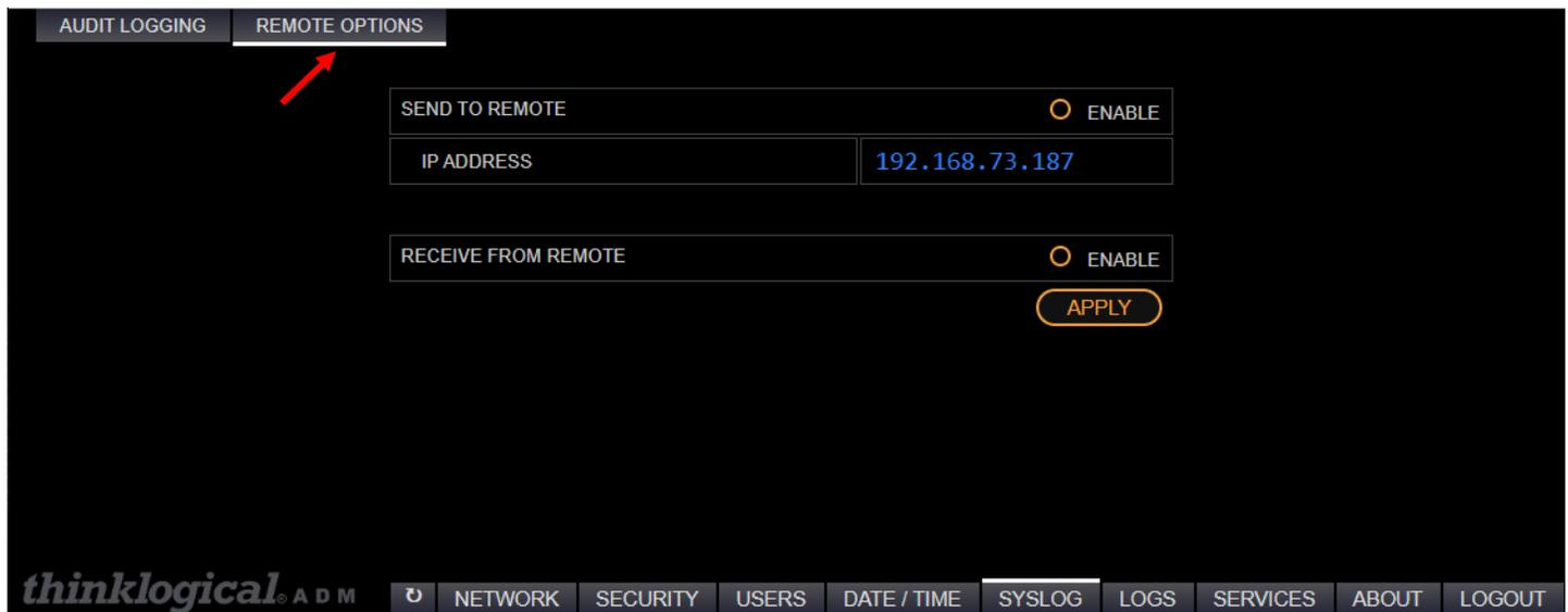
**SEND TO REMOTE – ENABLE:** Sends SYSLOG messages to a centralized logging server located at <IP ADDRESS> utilizing UDP/IP port 514.
