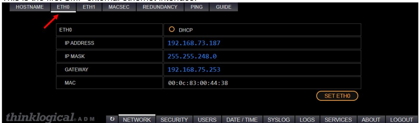
**[DHCP]** – Enables SMP to obtain IP address, mask and gateway from a “Dynamic Host Configuration Protocol” server.
