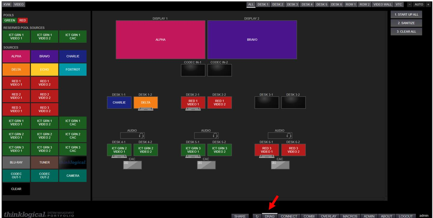
Connections are made by dragging a SOURCE icon from the POOL or SOURCE frame (or from another Destination) to a desired Destination. The Keyboard icon indicates which Destination has control of the keyboard. In this example, DESK 3-1 has control of the keyboard for Source CHARLIE.
