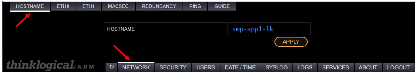
**HOSTNAME** - Defines the name of the Linux machine. Hostname is mapped to an IP address via “hosts” file or a Domain Name System (DNS) server.
