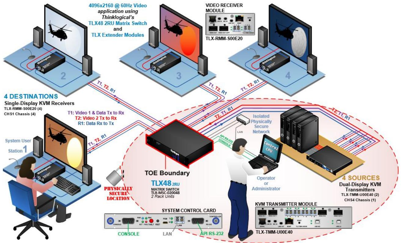
**Figure 2b. Typical TOE TLX48 2RU Matrix Switch Installation**
