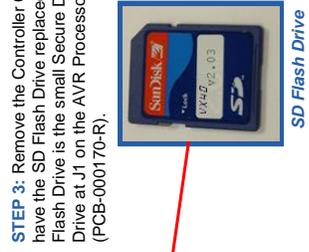
**STEP 3:** Remove the Controller Card that will have the SD Flash Drive replaced. The SD Flash Drive is the small Secure Digital Memory Drive at J1 on the AVR Processor Board (PCB-000170-R).
