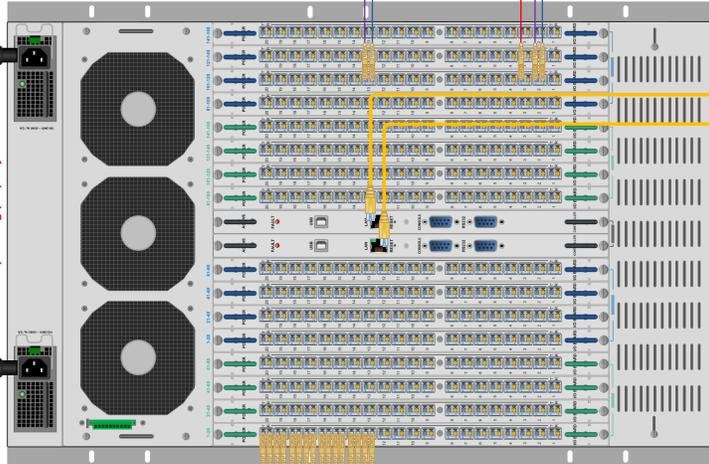
VX160 Router KVM Matrix Switch Chassis
