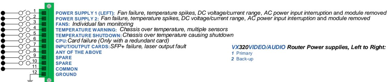
The VX320 Matrix Switches Critical Hardware Alarms:
