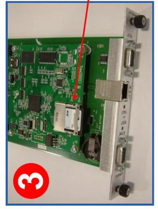
**STEP 4:** To eject the SD Flash Drive from its connector bracket at J1, press the exposed edge of the card into the bracket. A spring-latch will release and eject the SD Flash Drive. The new SD Flash Drive can now be inserted into the J1 connector bracket until it snaps into place.
