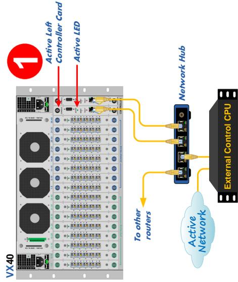
**STEP 1:** To replace the SD Flash Drive on a VX40 or VX80 Controller Card it is not necessary to power down the router if both Controller Cards are installed and connected to an active network.
