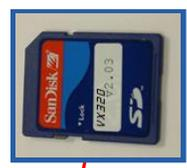
**STEP 4:** To eject the SD Flash Drive from its connector bracket at J1, press the exposed edge of the card into the bracket. A spring-latch will release and eject the SD Flash Drive. The new SD Flash Drive can now be inserted into the J1 connector bracket until it snaps into place.
