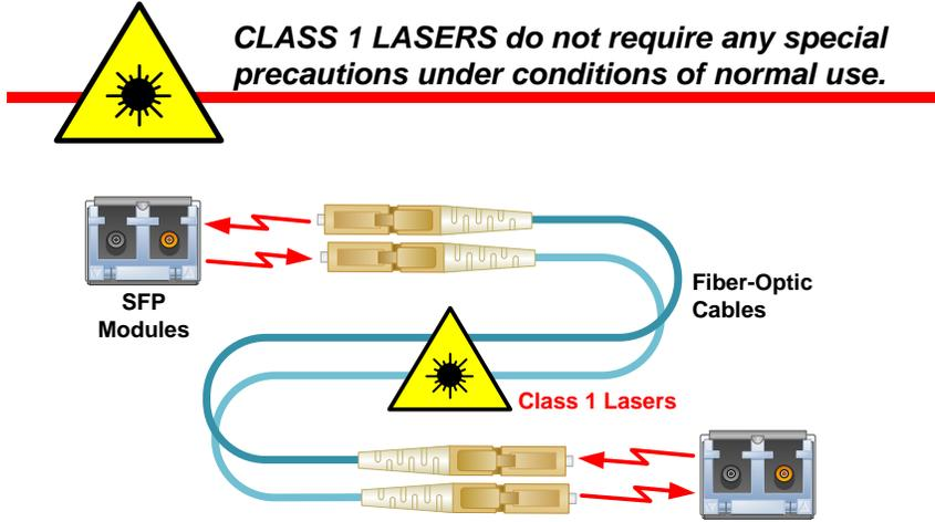
Unlike copper cabling, fiber optic cable requires special handling. A small bit of dust or a scratch on the ferrule tip can attenuate the optical signal so that it becomes unusable.
