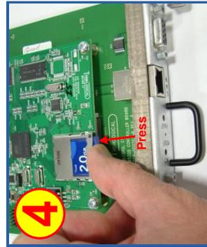
**STEP 4:** To eject the SD Flash Drive from its connector bracket at J1, press the exposed edge of the card into the bracket. A spring-latch will release and eject the SD Flash Drive. The new SD Flash Drive can now be inserted into the J1 connector bracket until it snaps into place.
