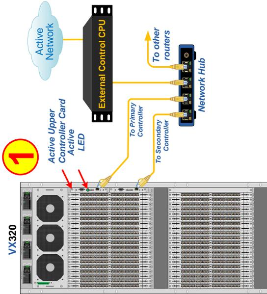
**STEP 1:** To replace the SD Flash Drive on a VX320 Controller Card it is not necessary to power down the VX320 if both Controller Cards are installed and connected to an active network.
